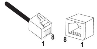
Figure 43. RJ-45 Connector and Port Pin Layout
